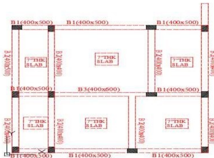
Fig-6: showing beam layout of the structure
